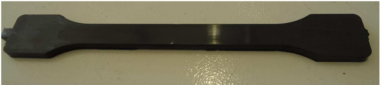
Figure 5.9 - Tensile specimen moulded by RHCM process.
