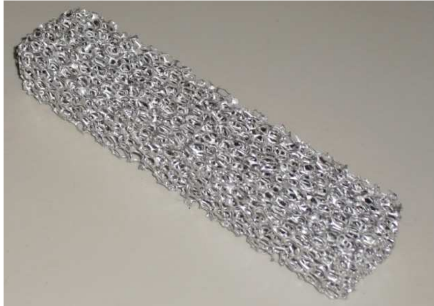
Figure 4.1 - Open-cell aluminum metal foam sample.
