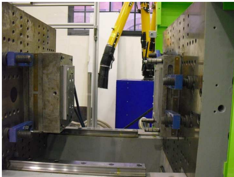
Figure 5.5 - The mould for tensile specimens with the new insert.
