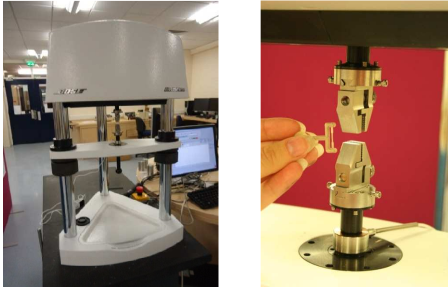
Figure 9.10 - Bose Electroforce 3200 test instrument (left), with tensile jaws and a moulded specimen (right).
