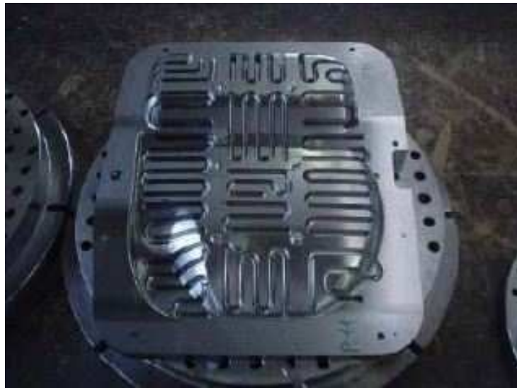
Figure 2.16 – An example of RHCM mould with conformal cooling channels.
