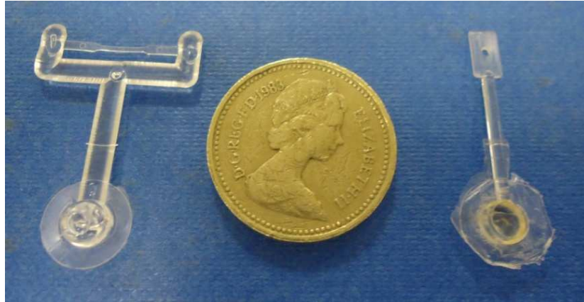
Figure 9.7 - Components chosen for the weld line study.
