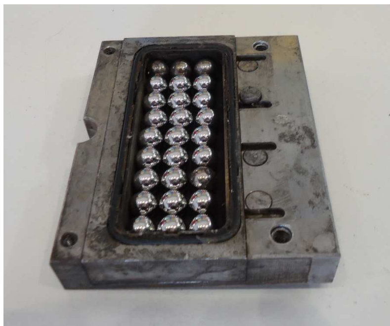
Figure 8.6 – Fixed insert with ball filling.
