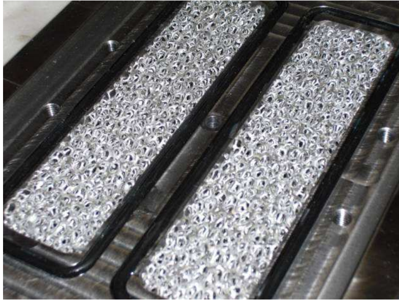
Figure 5.4 - Cavity with aluminum foam.
