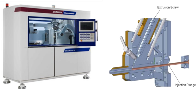
Figure 5.48 On the left: Wittman Battenfeld Micropower 15; on the right: Injection moulding unit
