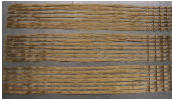
Figure 41. PBO fiber net after removing the transversal bundles.
