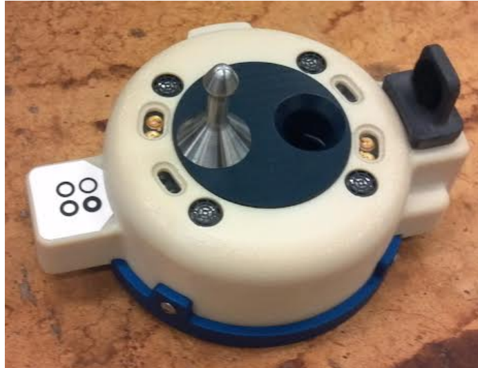
FIGURE 1.13: SPHERES Universal Docking Port
