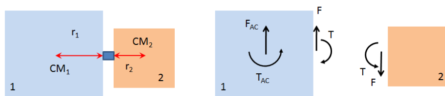
FIGURE 3.3: Load transfer model: docked spacecrafts geometry (left) and loads on the docking ports (right)
