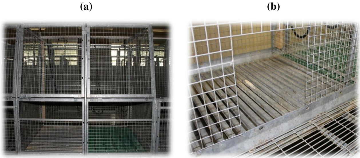
Figure 4.1. Open-top collective pen consisted of two modules (a) connected to each other by a hole (b).
