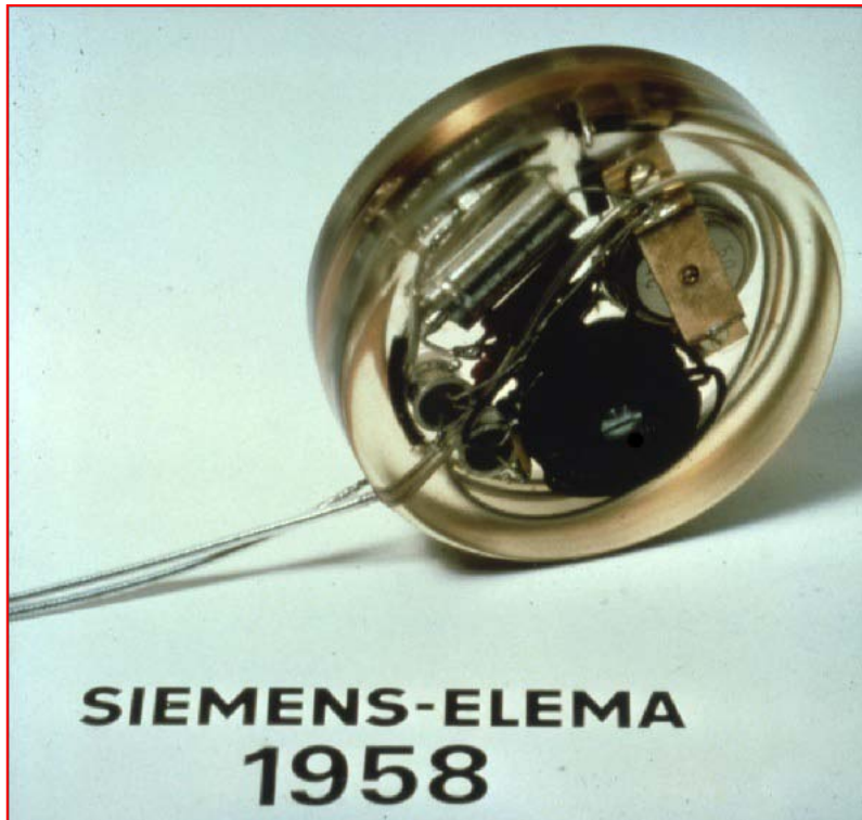
Fig 1 B: First miniaturized subcutaneous implantable epicardial pacemaker (Dr. Senning, Karolinska Institute, Stockholm Sweden, October 1958)
