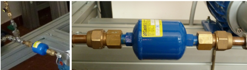
Figure 4.31: Picture of the filter and of the refrigerant charge port.
