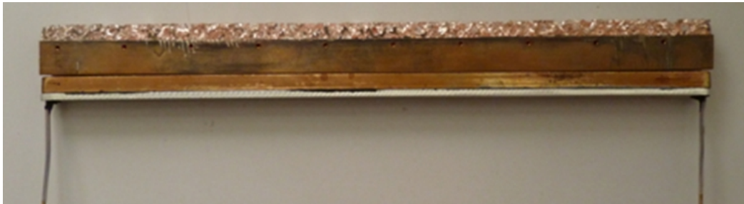
Figure 4.41: Picture of the electric heater.
