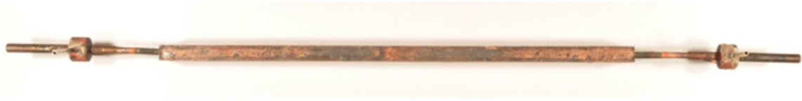
Figure 6.2: Picture of the tested microfin tube brazed in the copper heater.
