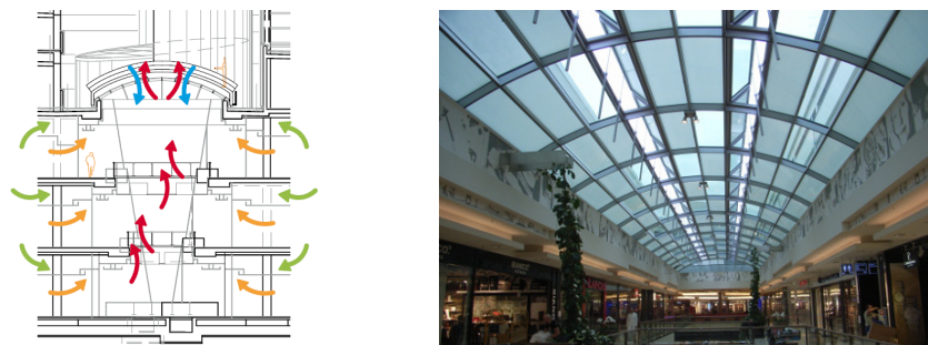
Figure 8 Ventilation concept ( left) and a detail of the gallery roof openings ( right) for the Ernst-August-Gallerie Source: Window Master
