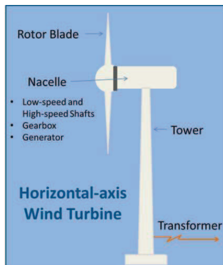
Figure 2.8: Basic parts of a wind turbine.
