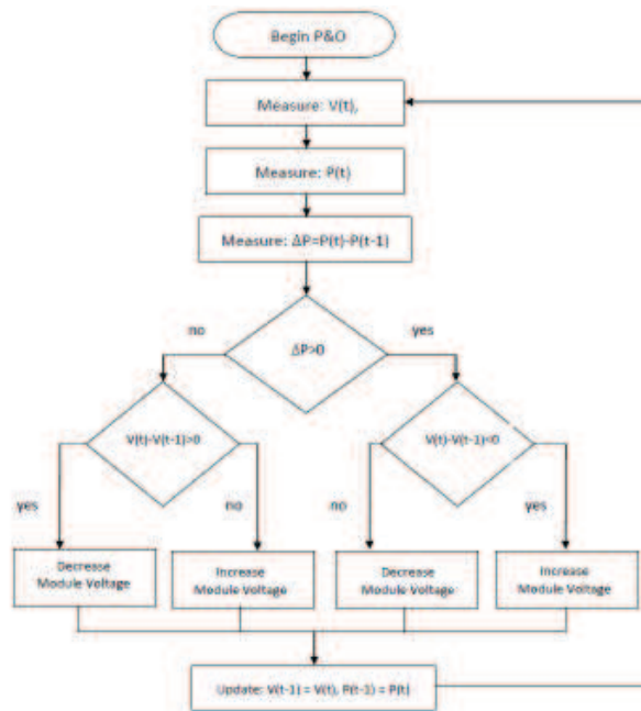
Figure 3.18: A flowchart of the perturb and observe MPPT algorithm.
