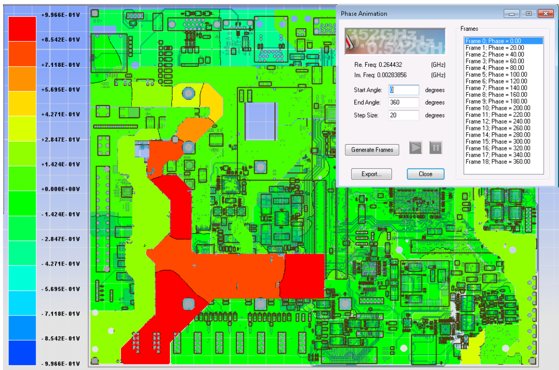
Figure 3.16: Voltage distribution between PWR6 and GND8 induced by the resonant mode 3 that occurs at 264 MHz.
