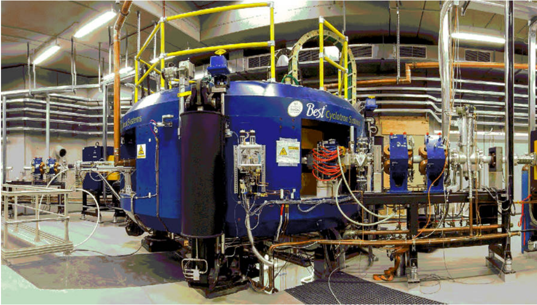
Figure 1.4: The 70 MeV cyclotron installed at LNL.
