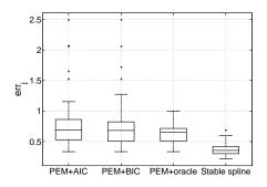
Fig. 5. Model selection example (Section 6.3). Boxplots of errors  $err_j$  (see eq. (32)) relative to the 4 estimators used to reconstruct the Runge function reported in eq. (36)
