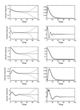
Fig. 3. Discrete-time test functions (Section 6.1). Results from Monte Carlo simulation using white noise as system input: true impulse response (solid line) and 99% variability bands of the estimates (dashed lines) obtained modeling the unknown function using the classical cubic spline kernel W (left) and the stable spline kernel K (right)
