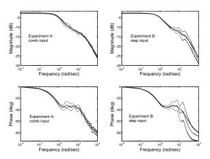
Fig. 8. Continuous-time second-order system (Section 6.4). *Top:* True magnitude Bode plot (thick line), nonparametric estimate (continuous line) and 99% confidence intervals (dashed lines). *Bottom:* True phase Bode plot (thick line), nonparametric estimate (continuous line) and 99% confidence intervals (dashed lines). System input is a comb (left panels) or a step (right panels).
