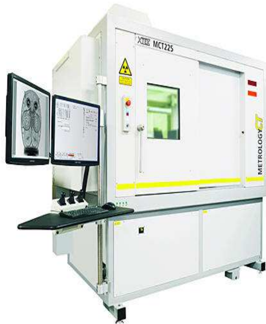
Figure 2.14 Nikon Metrology X-Tek MCT225 ® metrological X-ray Computed Tomography system.
