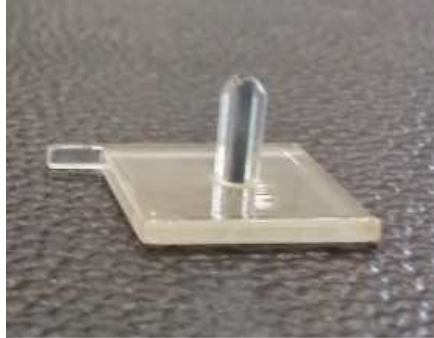
Figure 7.5 3D printed container with a diameter of 1.5 mm and a height of 10 mm.
