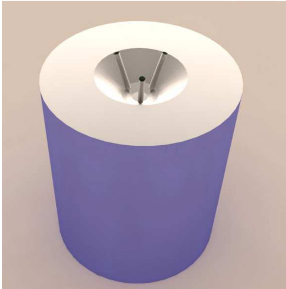
Figure 8.1 Concept of the new deposition nozzle: domain of the Argon-powder mixture inside the feeding pipes and sintering chamber of the micro DLMD-machine.
