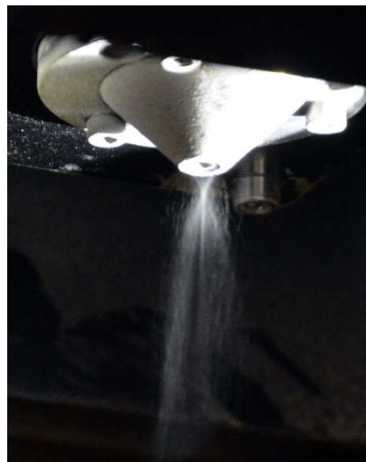
Figure 2.8 Powder cone coming out from the deposition nozzle.
