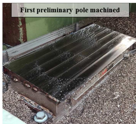
Fig. 4.46. First preliminary pole machined at the LNL.
