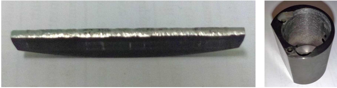
Fig. 3.70. Anodize aluminium paddle and ruined stator chamber after the tests.
