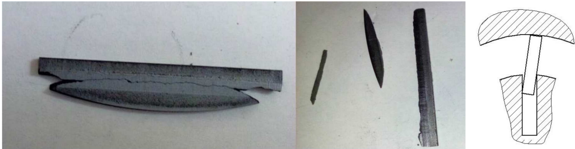
Fig. 3.68. Pictures of the broken graphite paddles and main wear mechanism leading to rupture.
