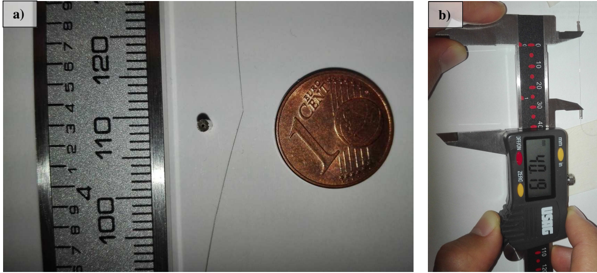
Fig. 3.41. a) Example of the capillary tube with a 50 \mu\text{m} diameter wire; b) test of the wire block precision.
