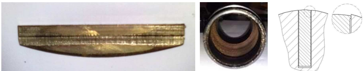
Fig. 3.69. Picture of the bronze paddle, the stator chamber and the wear mechanism leading to the motor block.
