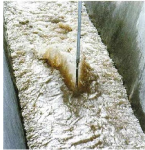
Figure 21: Turbidity meter at the outlet channel of the Rio Cordon Monitoring station.
