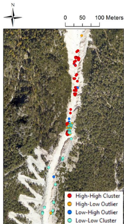
Fig. 2.6: Local Moran's I index map of the thin-plate spline function absolute errors at the spatial resolution of 1.00 m. Note the local clusters of high and low errors values, mainly located along the upper part of the channel where the topographic roughness is higher due to the presence of boulders and bank failures. Moreover, local outliers concentrate near the rock step at an altitude of about 1 500 m a.s.l..
