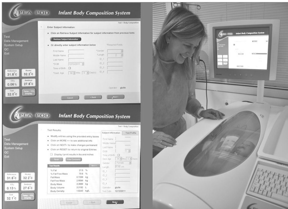
Figure 12. Left: ADP system monitor showing the initial screen (top) with required fields and the output screen (bottom) with body composition measurements. Right: a baby and her mother during volume measurement.
