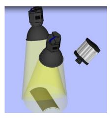
**Figure 1.1:** Infrared thermographic inspection: the known surface is heated with a flash, and experimental temperatures are collected through a thermographic camera.
