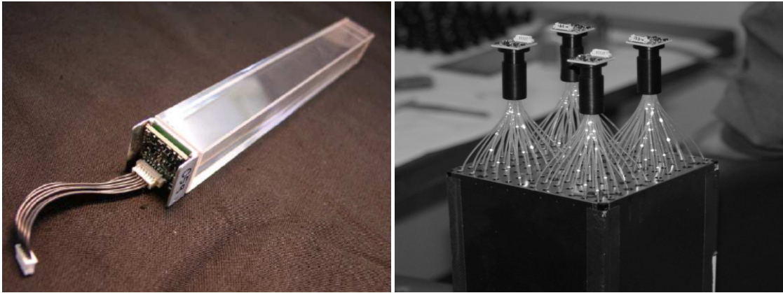
Figure 2.11: Left panel: Crystal detector unit of the PHOS detector. Right panel: Prototype of EMCal module.
