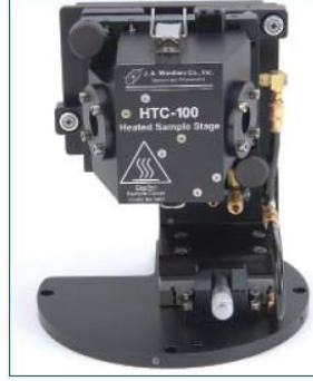
Fig. 40: Picture of a Woollam HTC-100 chamber, mounted on its stage.
