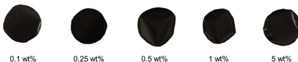
Figure 3-17: Images of the five types of CNH-PhOMe@PLLA composites having different concentrations of nanofillers in the polymer phase.
