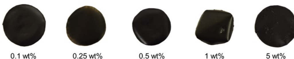
Figure 3-13: Images of the five types of MWCNT-PhOMe@PLLA composites having different concentrations of nanofillers in the polymer phase.
