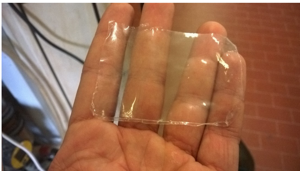
Figure 2-19: Image of the PLLA film used to prepare our first implant prototype.
