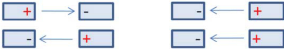
Figure 3-8 Electric dipole induced by the current distribution. (a) Anti-symmetric current distribution, (b) symmetric current distribution
