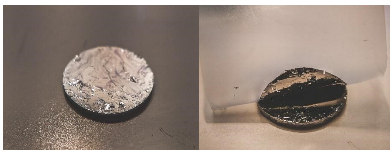
Figure 3.14. a) ruined HOPG surface before cleaving; b) scotch tape removal of a thin layer of graphite to expose a freshly cleaved HOPG surface.
