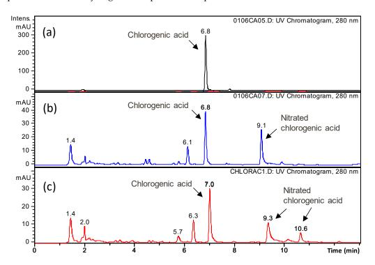
**Figure 6.** UV chromatograms (280 nm) of (**a**) untreated, (**b**) electrospray system (ES)-treated and (**c**) batch system (BS)-treated chlorogenic acid solution ( $5 \times 10^{-5}$  M) in the phosphate buffer (21.6 mM, pH 3.2).
