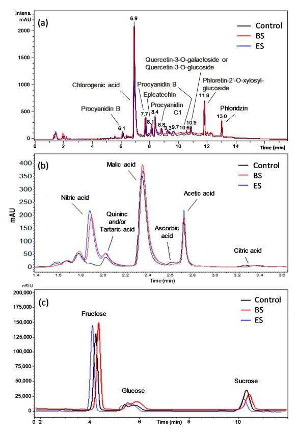
**Figure 5.** HPLC analyses of the untreated (control), batch system (BS)-treated, and electrospray system (ES)-treated apple juice samples using instrumental conditions to detect (**a**) polyphenols, (**b**) organic acids, and (**c**) sugars (see the Material and Methods, Section 2.5 for details).
