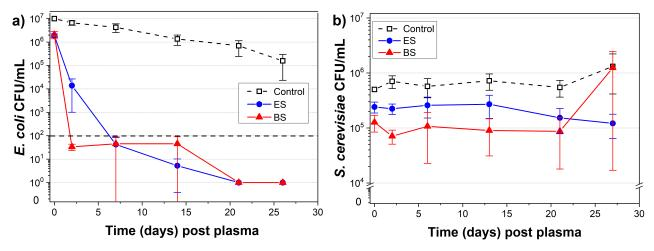
**Figure 8.** The post-plasma-treatment evolution in the electrospray system (ES) and batch system (BS) of the inactivation rate of (**a**) *E. coli* bacteria and (**b**) *S. cerevisiae* yeast with a high initial load in the apple juice, shown as a logarithmic scale (mean  $\pm$  SD, n = 3). The dashed line in (**a**) represents the acceptable level of *E.coli* ( $\leq 10^2$  CFU/g) in unpasteurized fruit juices.
