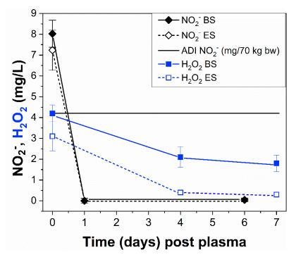
**Figure 2.**  $NO_2^-$  and  $H_2O_2$  concentrations (mean  $\pm$  SD, n = 3) that was measured in the air-transientspark-treated fresh apple juice compared to the ADI dose ( $NO_2^-$ ), which was calculated for a human with a 70 kg body weight. The shown measured and ADI values are directly comparable assuming the daily consumption of 1 L of the juice per person.
