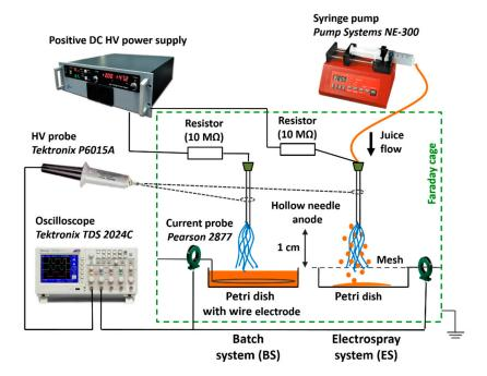
**Figure 1.** Experimental set-up of air transient spark discharge in batch (BS) and electrospray (ES) systems for juice treatment.
