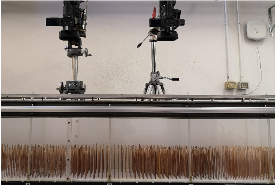
Figure 3.1 The experimental apparatus: side view of the test section with the array of cylinders in the most dense pattern and the two fixed mounted cameras; the flow is from left to right.
