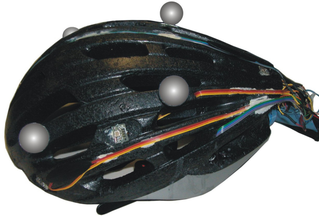
Figure 1 \alpha -prototype of the instrumented helmet
