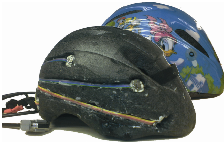
Figure 2 \beta version of the instrumented helmet
