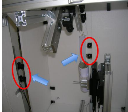
Figure 6.6: The inclined-can experiment setup. It is shown a can with markers, the two stereo-pairs and the positioning robot.
