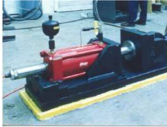
Figure 2.36 – MR damper 20 ton for civil applications.
