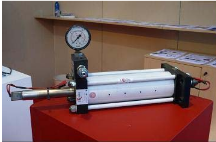
Figure 4.10 – Double ended 10 KN MR damper. (Photo by FIERA LAMIERA 2010).
