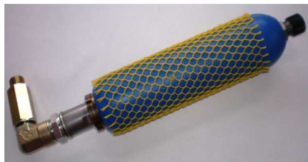
Figure 4.8 – Hydraulic reservoir of the damper for the volume change compensation.
