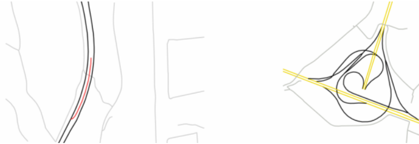
Figure 25: (left) an error in the classification of the input data is detected: the edge classified as highway (red) is too short to be a highway and, as a slip road, it is not connected to anything; it will then not be considered part of the highway. (right) The classification of slip roads and carriageways is reliable also in complex cases.
