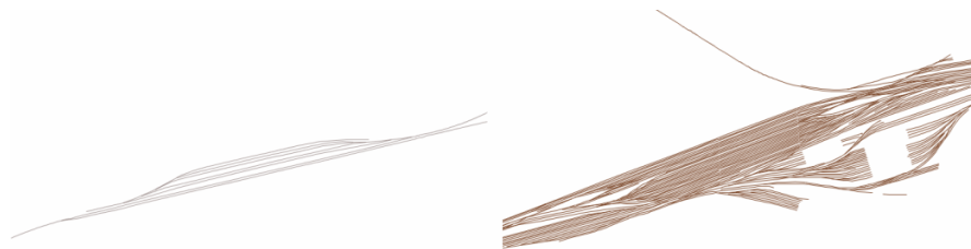
Figure 46: example of different complexity in the source 1:5000 data; a simple case comprising only 27 elements (left) and a complex case comprising 288 elements (right).
