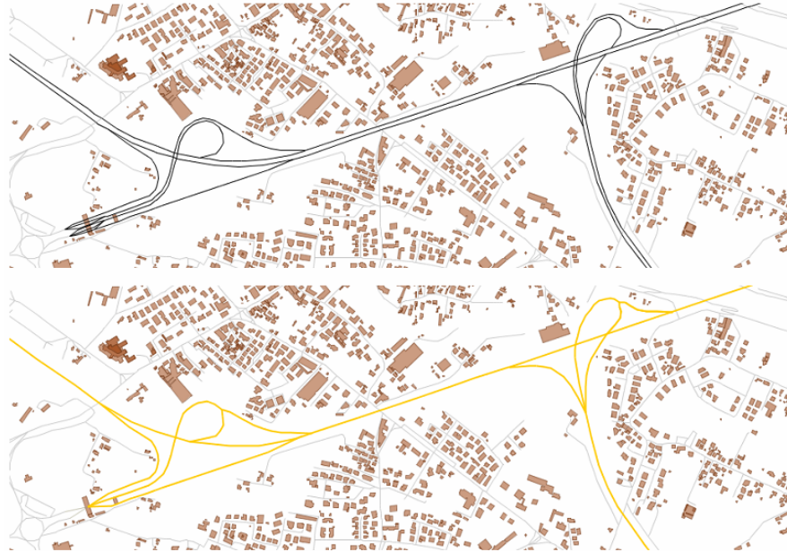
Figure 50: results of the generalization of the highway: original data (top), generalized data (bottom); it is possible to observe how the dual carriageways have been collapsed to a single line, how the slip roads have been connected to this new line and how the toll-plaza (bottom left corner) had been simplified.
