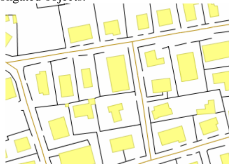
Figure 7: fences (black lines) in a urban context (buildings in yellow, roads in brown); according to IGMI specifications, a gap smaller than 10 m in a fence should be ignored and the fence derived as a continuous line
