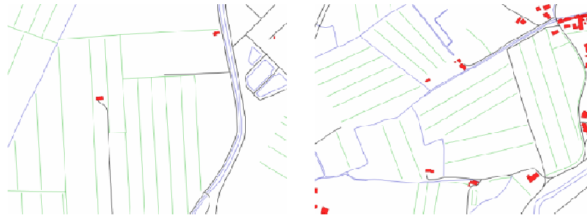
Figure 32: on the left ditches connected to other hydrography features, on the right ditches not connected; the latter type is the most frequent.
