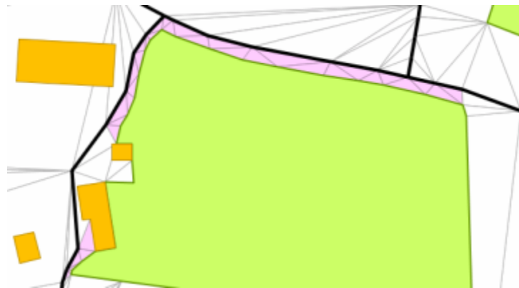
Figure 38: the extension of the boundary of a wood patch using the CDT (gray lines); woods are in green, roads in black: the pink triangles are those selected to be merged to the wood to extend its boundary; a threshold on the height of the triangles is used to select the triangles. Overlaps between buildings (orange) and woods are allowed by the specifications.
