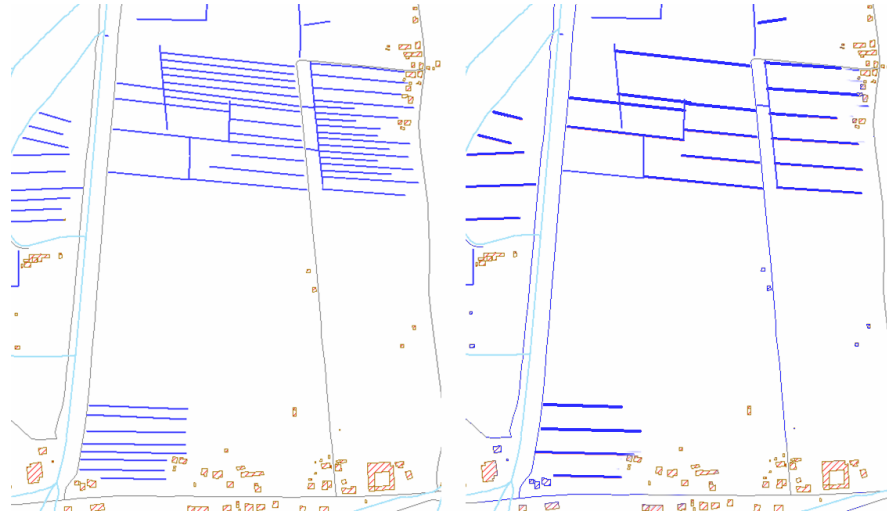
Figure 52: generalization of ditches: before (left) and after (right); the number of ditches has been greatly reduced, while the patterns have been maintained.
