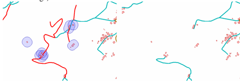
Figure 18: removing dangling edges. Left: in red dangling edges candidate to deletion (after the first iteration). Right: final result after the iterative procedure: all the dangling edges not leading to a group of buildings or being a redundant connection to them have been deleted
