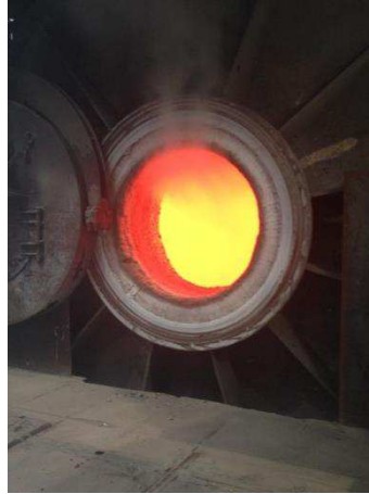
Fig. 2 Charging door of the rotary furnace used in the present work.
