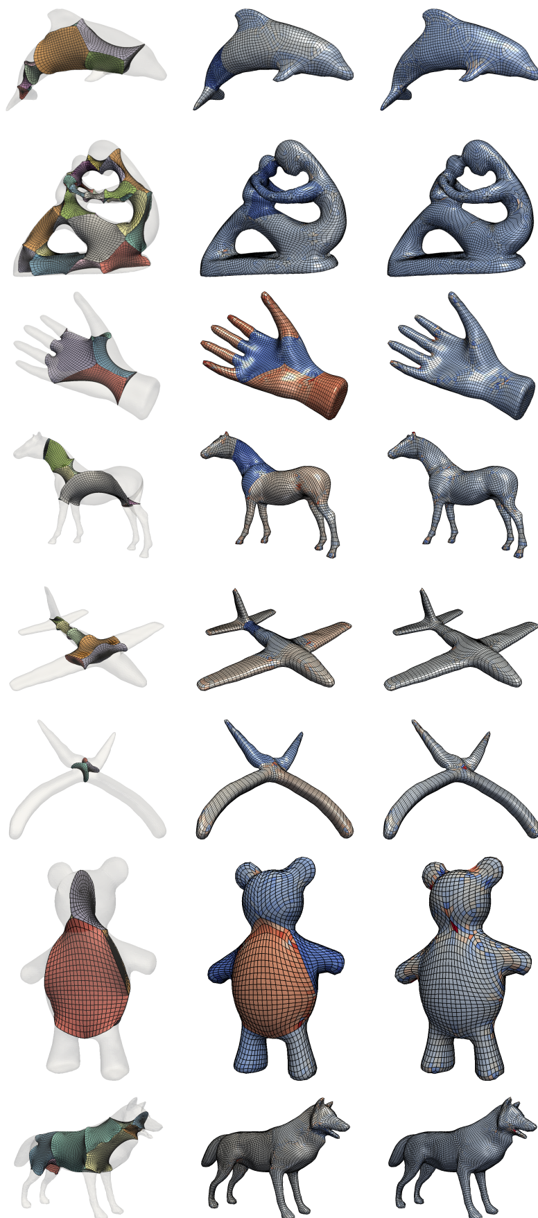
Fig. 7.6 Example 1: Reconstruction results of different meshes. from left to right: input skeleton S with outline of M_{\Delta} in transparent, result of ALG_1, result of ALG_2.
