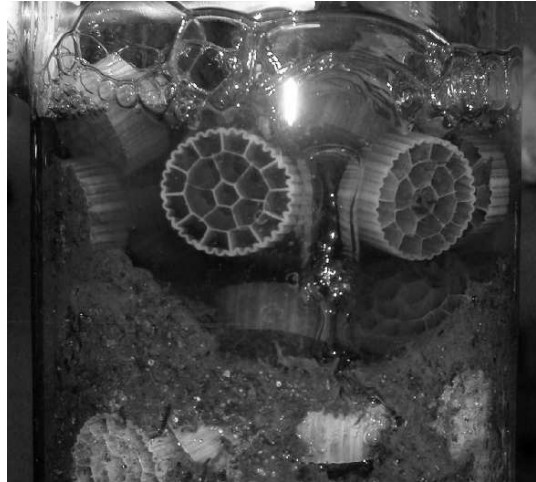
Figure 8.1: Example of flooding as consequence of an excessive bed compaction. Results obtained using 2:5 compos/inert carrier.
