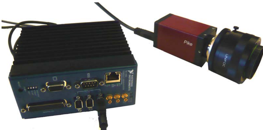
Figure 3.9 AVT™ PIKE camera connected to the National Instrument™ CVS-1455
