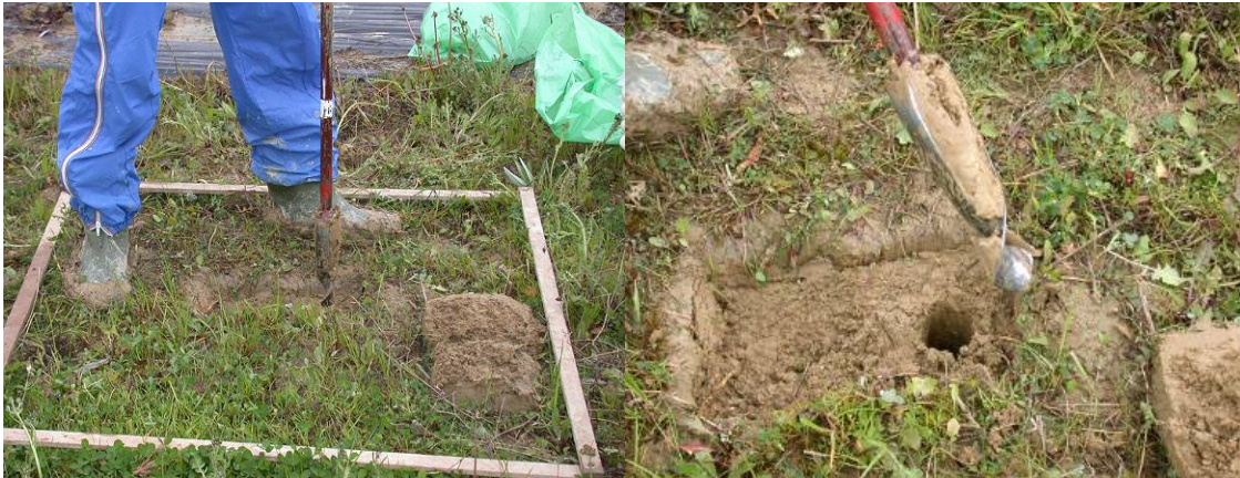
Fig. 5.2 – Soil sampling using a manual drill.
