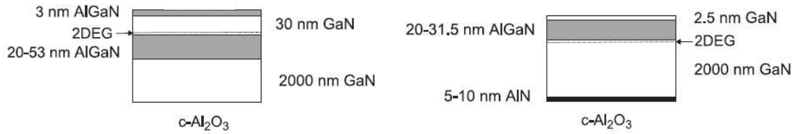
Figure 2.7: Study of the 2DEG localization on the basis of GaN face polarity
