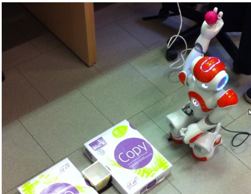
Figure 4.12: Overview of experimental scenario: the NAO is placed at 40 cm from the basket.
