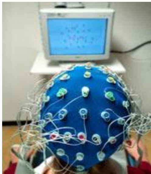
Figure 1.2. Example of a subject undergoing a non-invasive EEG acquisition.
