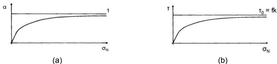
Figure 2.3. (a) Relative area of contact as a function of normal pressure. (b) General trend of friction stress versus normal pressure. [2]
