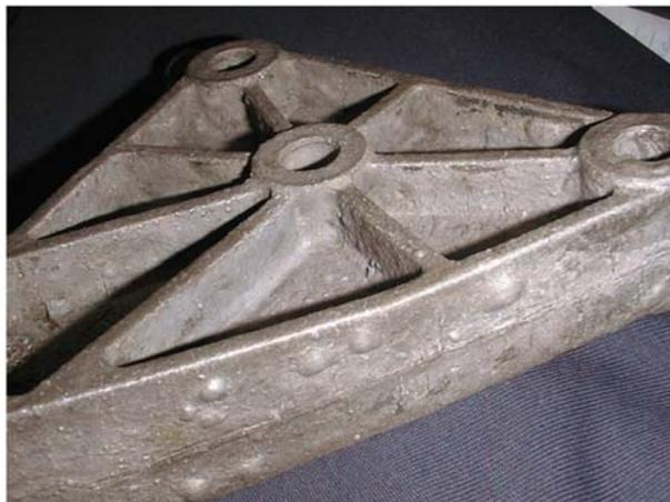
Figure 2.9: Blistering of HPDC casting after solution heat treatment.
