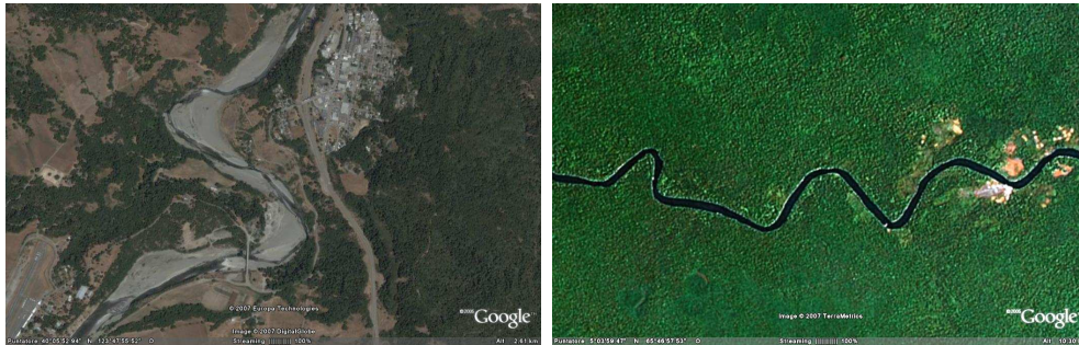
Figure 1: Meander bends showing the dependence of river width on curvature and stage. (a) Maximum widths experienced at bend apexes (Eel River, California) (from Google Earth); (b) minimum widths at bend apexes, and local widening in straight reach (tributary of the Amazon River, Brazil) (from Google Earth).
