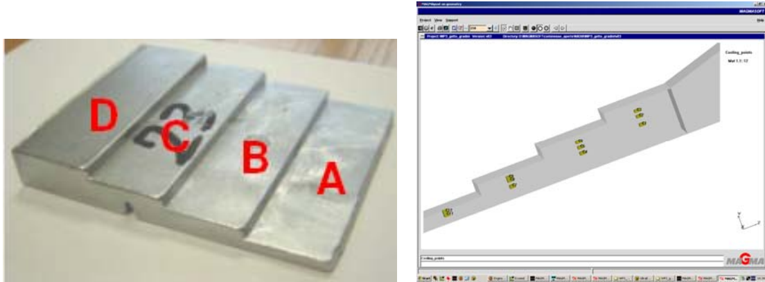
Figure 4: On the left, the reference step casting is shown while, on the right, it is illustrated the position of virtual thermocouples
