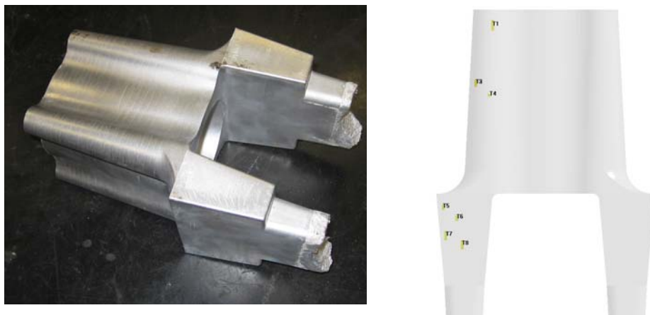
Figure 10: On the left, TKAL low pressure die casting mono-cylinder is shown while, on the right, it is illustrated the position of thermocouples.
