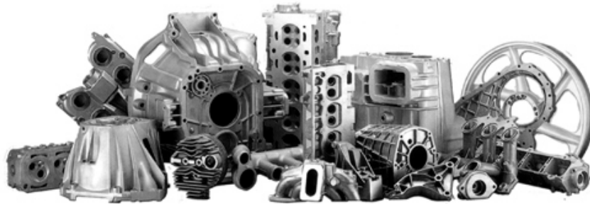
Figure 8. Examples of castings produced by means of the LPDC process.
