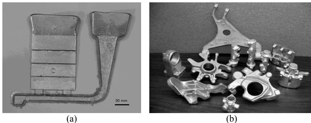
Figure 7. (a) Geometry of PMDC step casting used in Article 3 and Article 4 and (b) typical PMDC components.
