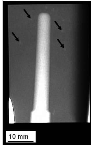
Figure 3. Radiographic image of the bulkhead support showing the presence of porosity.
