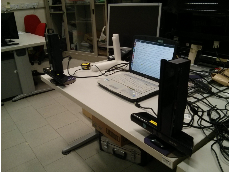
Figure 6.14: 3D DOA-ASL using four Microsoft Kinect setup.
