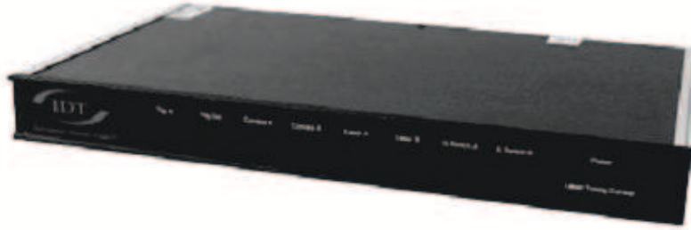
Figure 4.6: Terminal used in connecting PIV apparatus components
