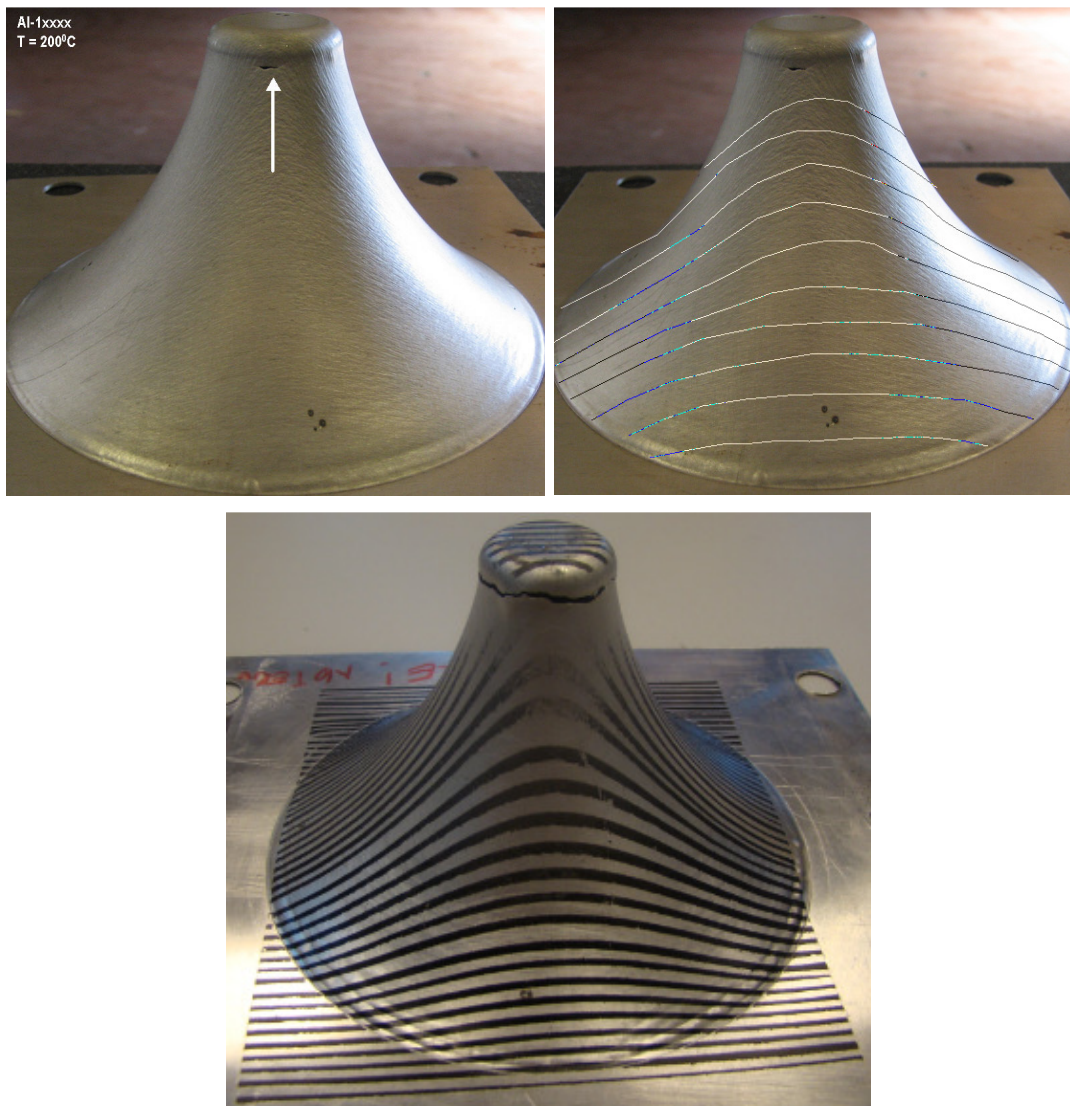
Fig. 3.17 The bell-shape propagation path of material flow
