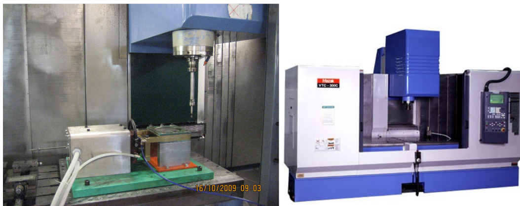
Fig. 3.5 MAZAK VTC-300C CNC machine using for SPIF process with metal sheet
