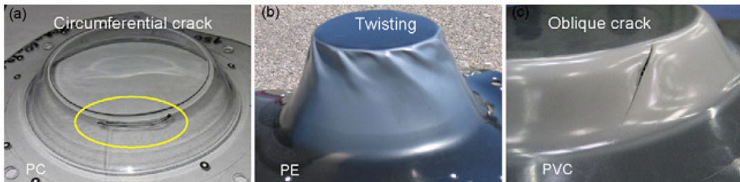
Fig. 3.23 Three different failure modes in PC, PE, and PVC [70]
