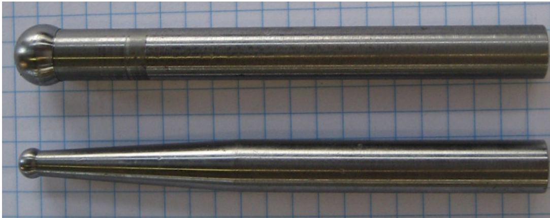
Fig. 3.2 Forming tools for SPIF process with polymeric materials
