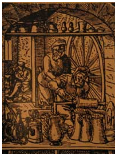
Fig.1.9 Wooden spinning with a manually operated flywheel [13]
