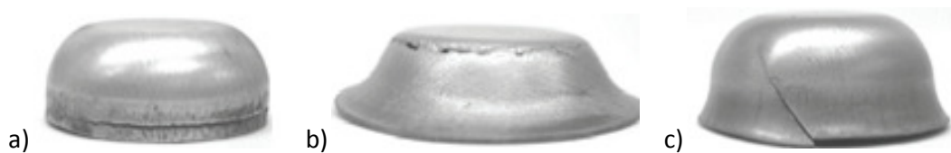
Fig. 2.2 Fracture of cold deep drawing
