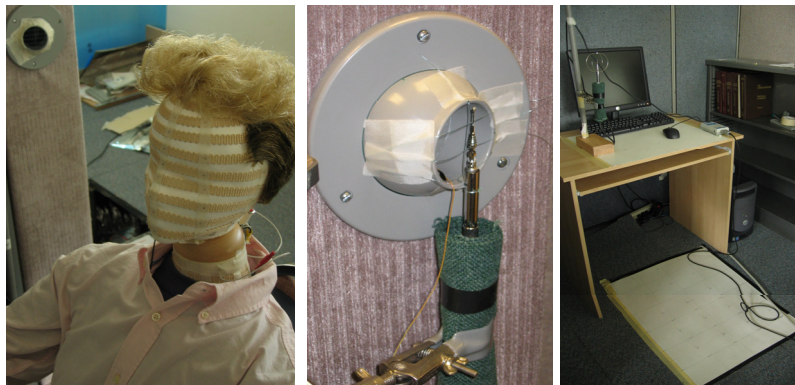
[Figures 2.47-2.49: Outlet and manikin, omni-directional sensor, measurement grid]
