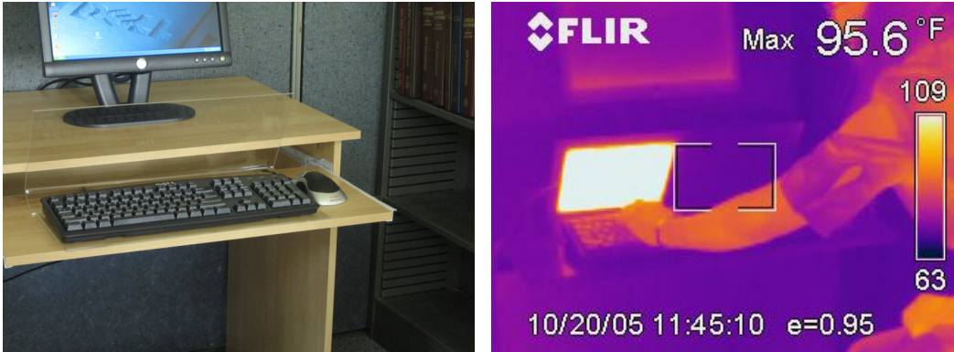
[Figure 2.14-2.15: Radiant hand-warming device. The clear screen with the thermal-clear heater]
