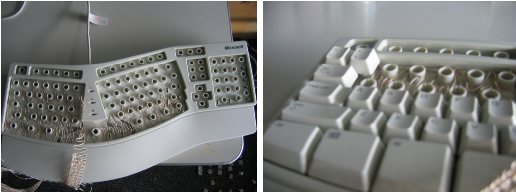
[Figures 2.16, 2.17: The resistance wire is applied between the keys and the topside of the keyboard.]
