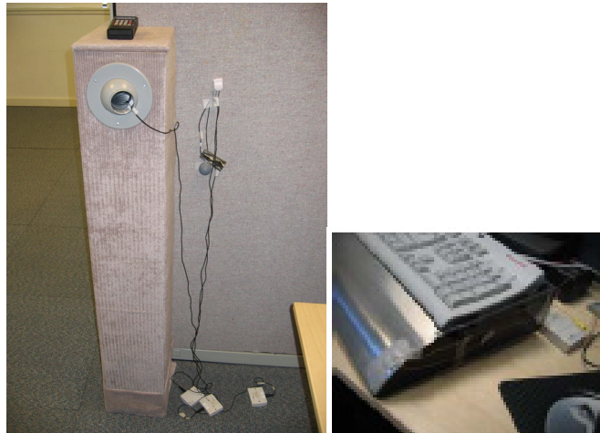
[Figure 2.63. Thermistors and thermocouple to measure workspace environmental conditions and the TAC system temperatures]
