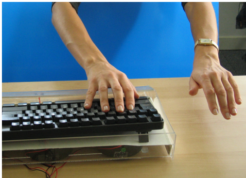
[Figures 2.33-2.38: keyboard and effect of the cool air. The left hand was not exposed to the hand-cooling device; the comparison between the two hands shows the effect of the device]
