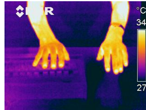
[Figures 2.33-2.38: keyboard and effect of the cool air. The left hand was not exposed to the hand-cooling device; the comparison between the two hands shows the effect of the device]
