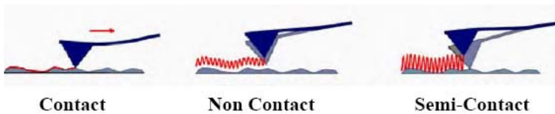
Figure 6. Scheme of the AFM working modalities. In contact mode the topography is obtained by the cantilever bending; in no- contact mode and semi-contact (or tapping) mode the signal comes from the variation of frequency, magnitude and phase of the cantilever oscillation.
