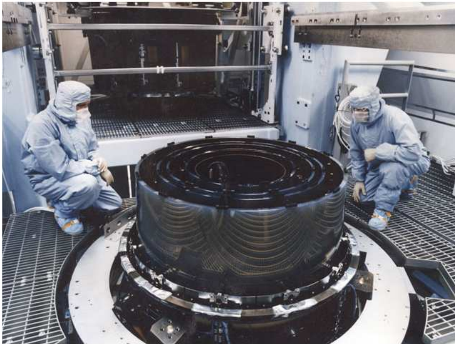
Fig. 6 Workers at Eastman Kodak in Rochester, N.Y., test the alignment of the Chandra observatory's High-Resolution Mirror Assembly. (font: www.nasa.gov/.../chandra/assembly.htm_prt.htm , photo of Eastman Kodak).
