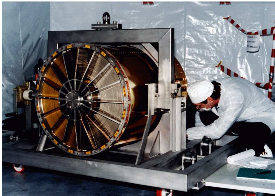
Fig. 7 One of the mirror modules from the XMM-Newton X-ray telescope. This module consists of 58 mirror shells made of gold-plated nickel. (font:
