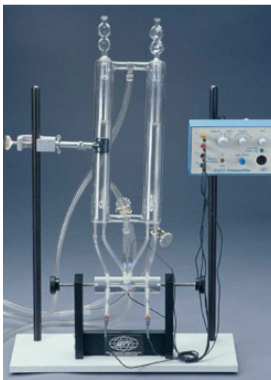
Fig. 2.5.3.1. Representation of the Ussing chamber technique, from http://www.warneronline.com/product_info.cfm?name=Introduction to Ussing Chamber and System from Warner&id=1401 .
