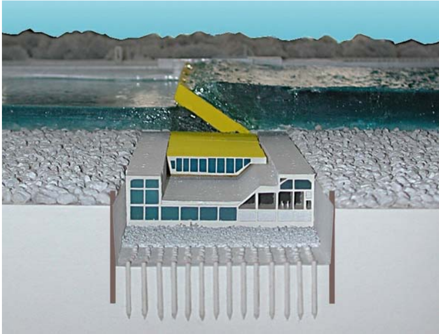
Figure 6.6:scheme of the movable gate in construction at the Lagoon inlets (www.salve.it)
