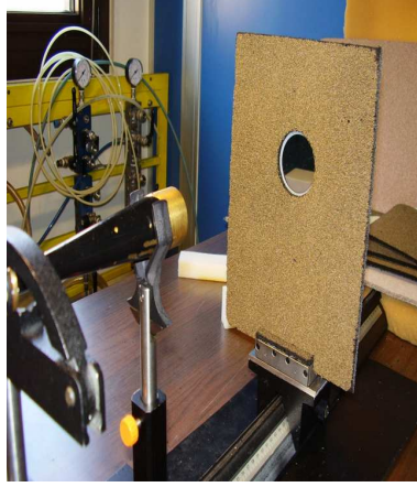
Figure 5.2: Picture of part of the calibration experimental setup (antenna and metallic mirror).
