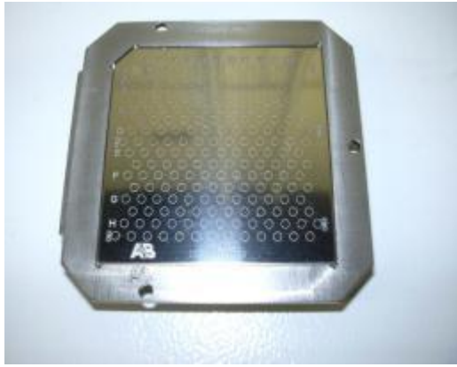
FIGURE 2-10 SAMPLE TARGET FOR MALDI.
